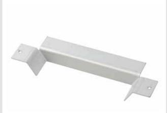
Material: galvanised steel 1.0 mm Dimensions: 144 x 41 x 15 mm Total number of bends: 5
