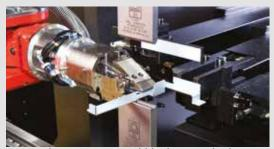
Robot can operate within the press brake
