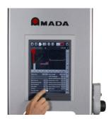
The NC control is capable of generating programs automatically. It takes into account bending constraints and ergonomics, including gauging position, component handling, bend order and required tolerance
