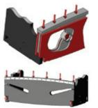
For higher tonnage versions the lower pins in the centre. This lower beam is secured to the machine frame by means of two pins in the centre of the lower beam, this allows for a certain degree of movement. Thus, when the cylinders exert the bending force at the extremities of the machine, the beam deflections are parallel.
