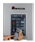
For special applications, manual mode programming allows the operator to create personalised programs.
