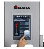
The operator enters the dimensions into a pop-up window. It is also possible to indicate bending priority.
