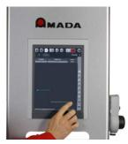
Drawings can be made directly on the NC by using the new touch-screen technology.
